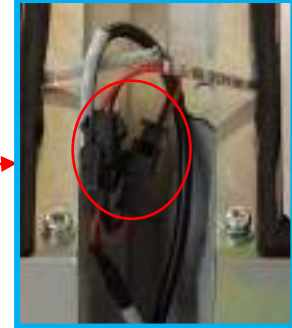
Power supply cable of left/right speaker assembly
