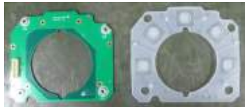
Trackball button board PCBA
