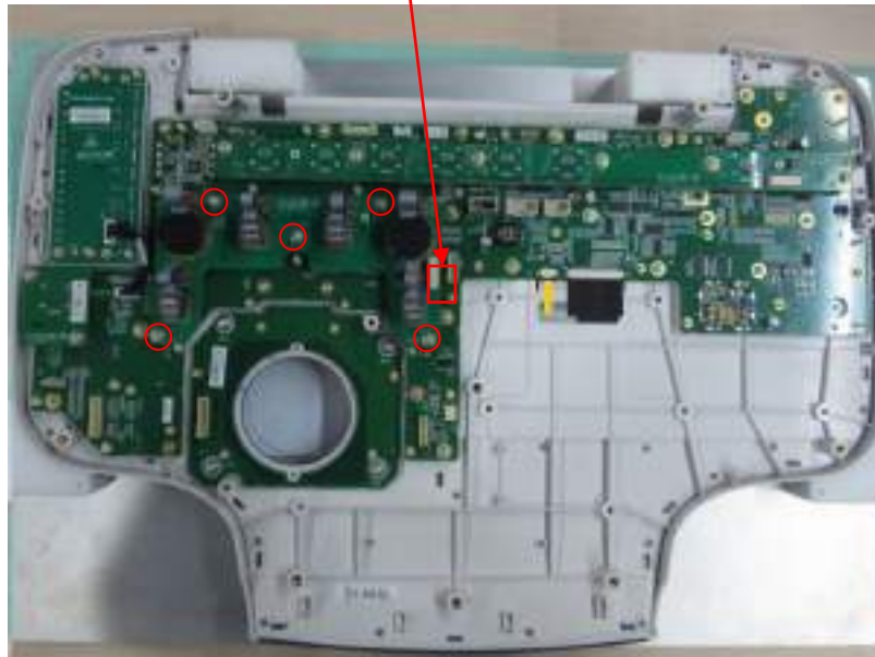
Multi-functional encoder board PCBA
