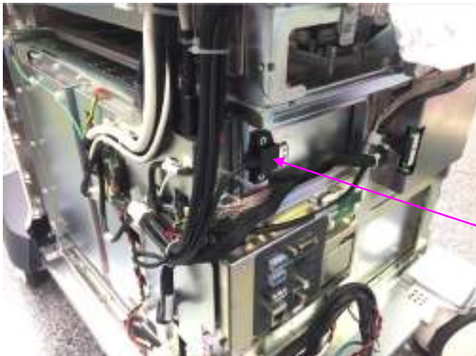
The flange of the backup plate is close to the Dongle and there is a tiny gap
