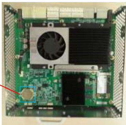
Button battery Lithium 3V 620mAh CR2450
