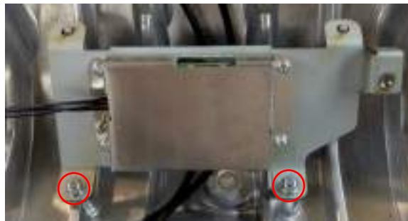
LCD signal connector PCBA assembly
